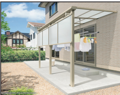
Up to 15' Projection, with Bearing Beam Maximum space between posts 18'
