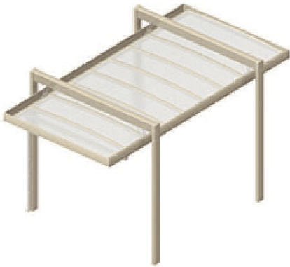
Roof Unit Suspended from Bearing Beams
